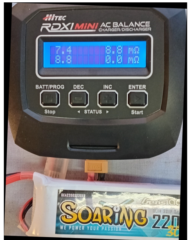
The Hitec charger can measure the resistance of the whole battery, and also of each individual cell.
