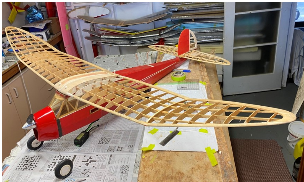
Left: The Clipper ready to cover. The big 72 inch wing is a thing of beauty
