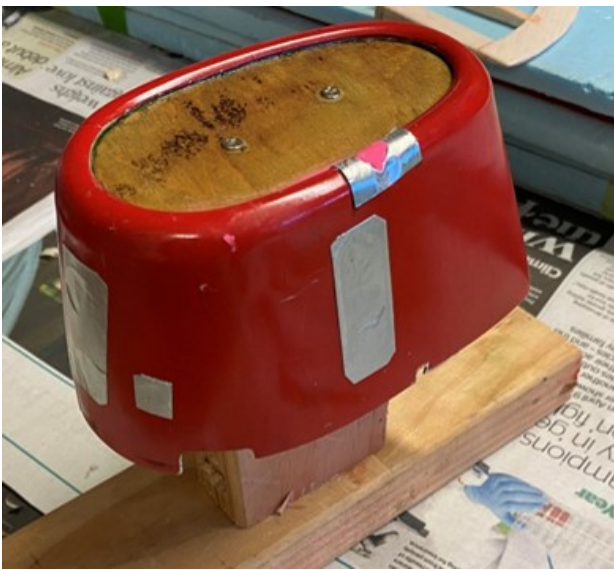
Above: Old plastic cowl prepared as a mould to glass over. Mounting on a stand helps a lot with handling.
