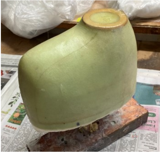
Styrene plug glassed with 2 plies of 4 oz and one of 2 oz using epoxy that doesn't attack the foam.
