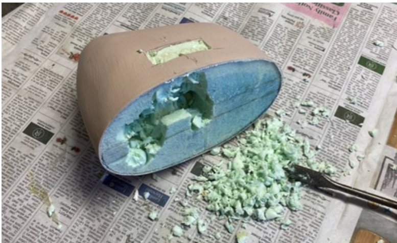
Styrene plug glassed with 2 plies of 4 oz and one of 2 oz using epoxy that doesn't attack the foam.
