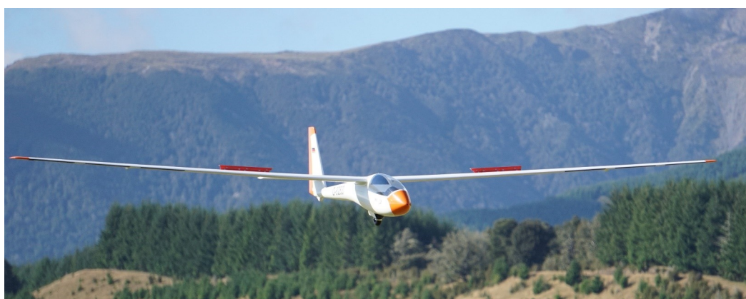
Typical St Arnaud background as Sam Laidlaw brings his 5m ASW15 (from Airworld Germany) in for a perfect landing. Crucifix tail is a neat but unusual set-up.
