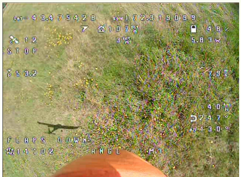
0.15 seconds before impact. You can see the flaps in the plane's shadow.
